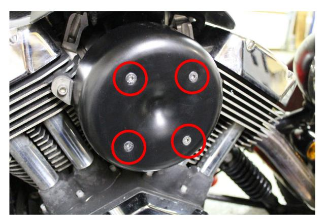
• Remove screws 4off (4mm allen key)
