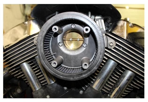
Check air filter is seated correctly on backplate
