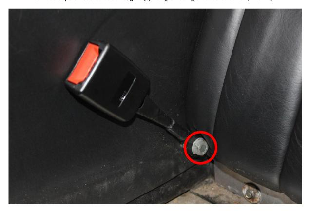
Remove buckle bolts (LH / RH) & buckles (17mm socket)
