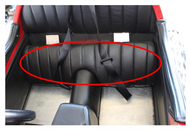
Remove lower rear rest (ease out from lower edge, careful not to bend brackets)
