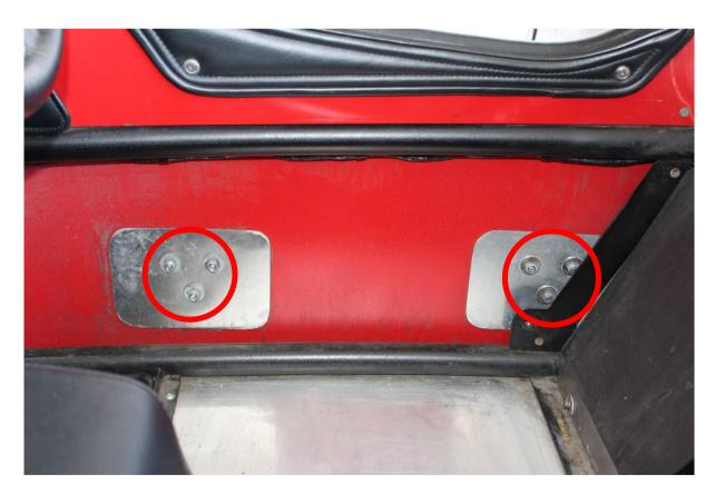
• Remove bracket nuts 3off (13mm spanner) & bracket (1x front and 1 x rear brackets)
