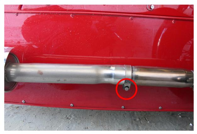
• Undo exhaust clamp (10mm spanner)
