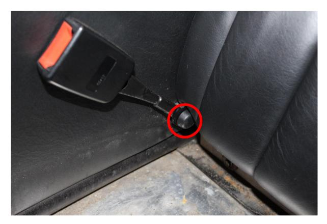
Remove caps on seatbelt buckle, gently prising off using a flat screwdriver (LH /RH)
